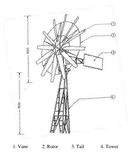
The reciprocating pump is fitted at 25 m. depth in a bore well. The vanes are reinforced with 25 x 25 x 8 mm. size L angles at the backside of the periphery for longevity.
